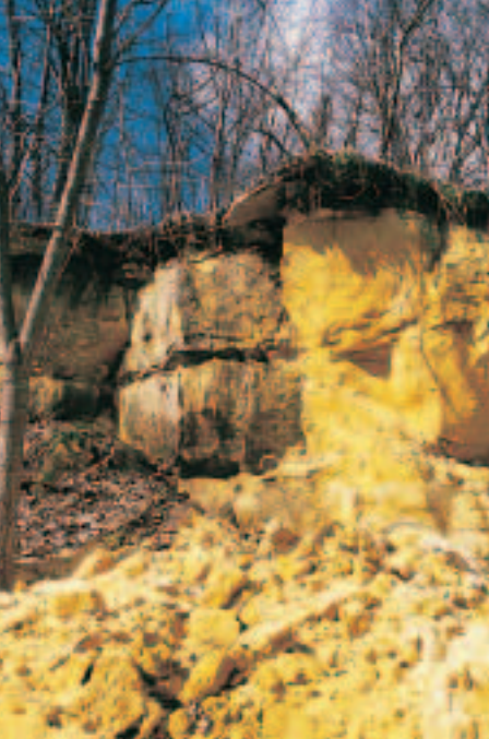
Figure 23-7 Glass is made from silica sand such as the very pure and clear St. Peter sandstone.
