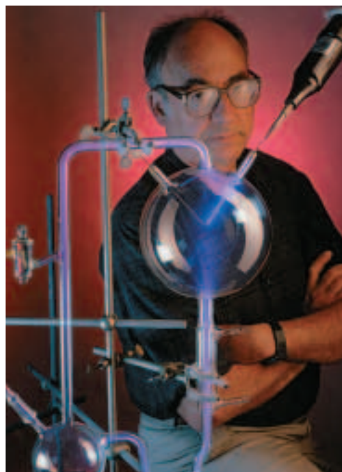
Figure 22-12 Dr. Stanley Miller is shown with a replica of the apparatus used to model Earth’s early atmosphere in the Miller-Urey experiment.
