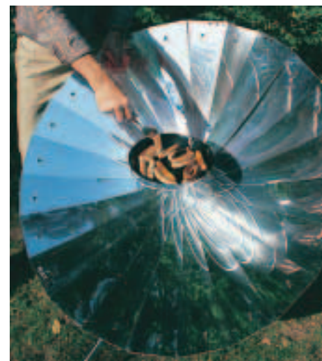
Figure 26-10 This parabolic solar cooker focuses sunlight on the spot where the cooking pot is placed.
