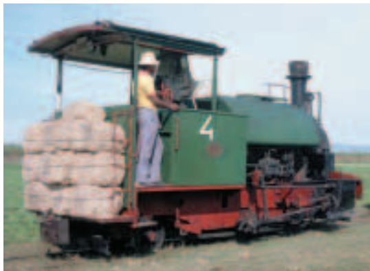
Figure 26-16 Bales of bagasse are burned to produce the energy that powers this steam locomotive in Java, Indonesia.
