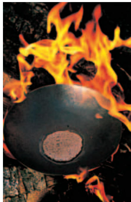
Figure 25-11 Small-scale miners in the Amazon River Basin use mercury to extract gold.
