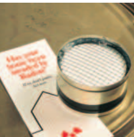
Figure 25-16 A radon test kit is a simple device that measures the amount of radon gas infiltrating a building over a week's time.
