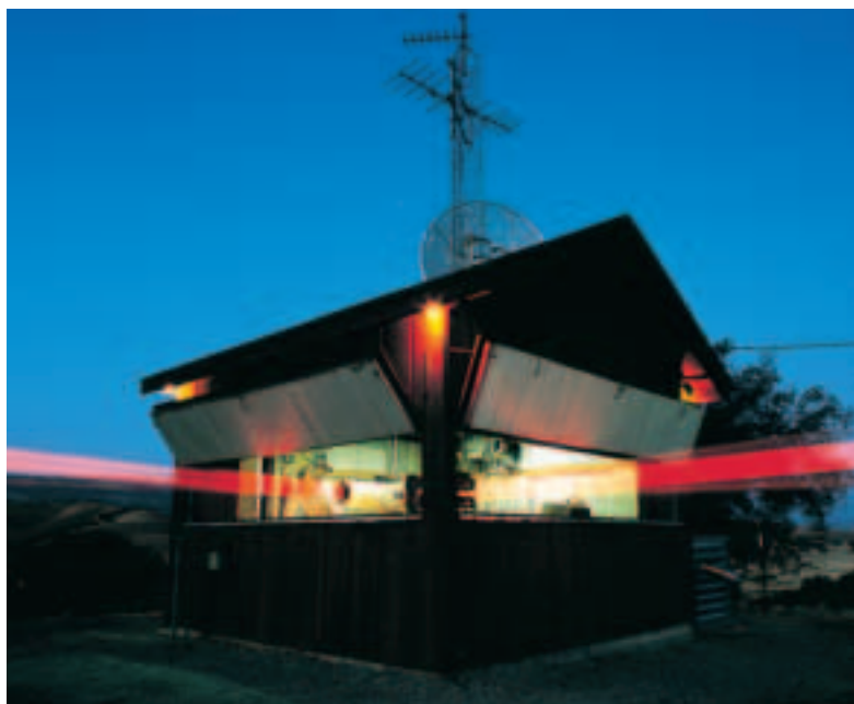
Figure 19-20 Lasers are just one technique being used to study earthquake probability in the area around Parkfield, California. Lasers can record very small movements along a fault.
