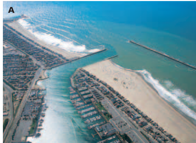
Figure 16-9 The entrance to Channel Island Harbor in Oxnard, California, is protected by jetties and a breakwater (A) . Jetties deprive downshore beaches of sand (B) . Breakwaters cause beach sand to accumulate and eventually close the anchorage (C) .
