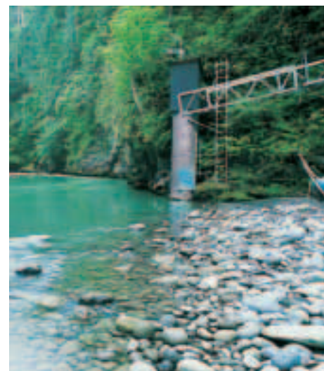
Figure 9-12 This USGS stream gauging station is located in the northwest section of Washington State.
