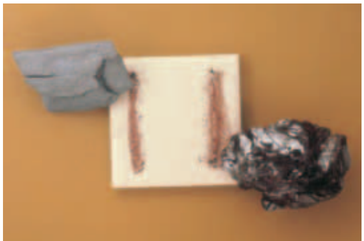
Figure 4-10 Both gray and black samples of hematite leave rust-colored streaks on a porcelain plate.
