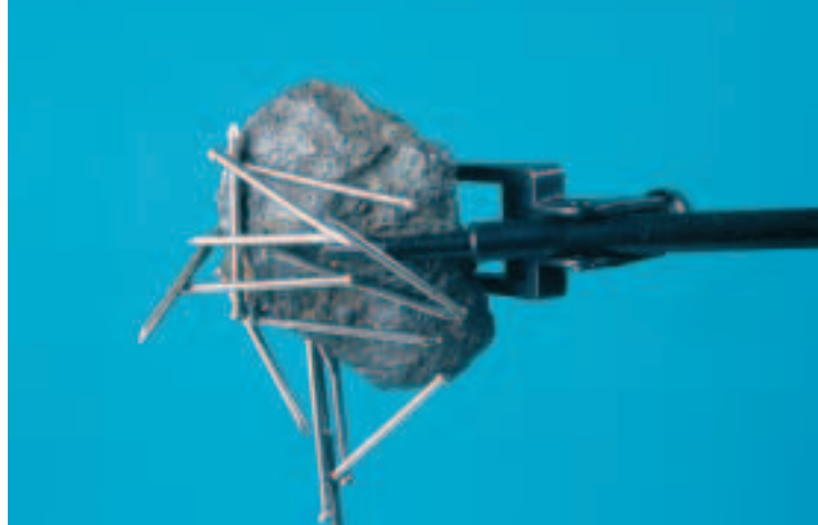
Figure 4-13 Magnetite can pick up iron nails because it is naturally magnetic.
