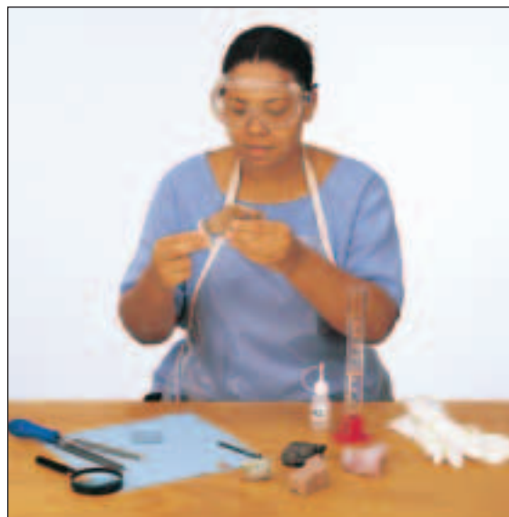
Figure 1-7 Safety goggles and a lab apron should be worn during any activity or experiment in the science lab.
